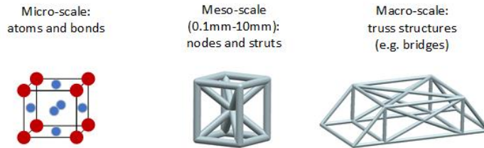
Figure 1: Scale levels of lattice structures, adopted from [27].
