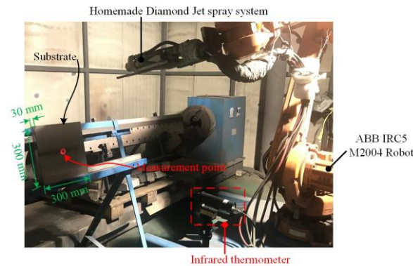
Figure 3: Experimental temperature measurement of the substrate surface.
