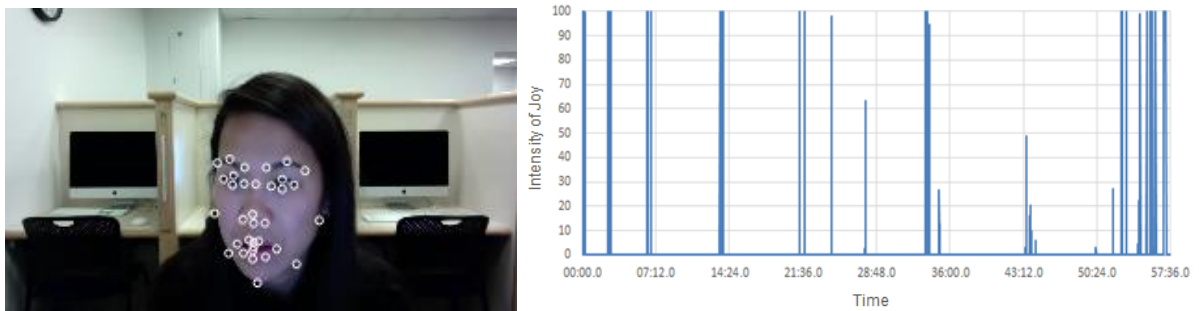
Figure 7: (Left) Emotion recognition algorithm showing points of significance. (Right) Data stream from sample video footage [28].
