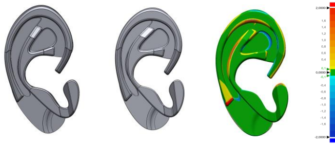
Figure 7: Map deviation resulting from the comparison of two surgical guides obtained in two iteration with two successive inputs of the same surgeon.
