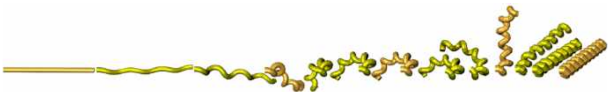
Figure 10: Sequence of large deformation shape generated from five helix shapes. Two frames (yellow) are inserted between two successive keyframes (orange).
