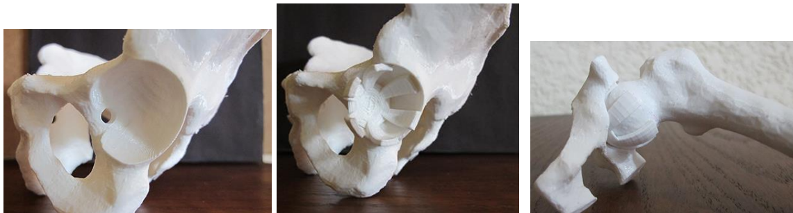
Figure 17: 3D prototype: (a) Pelvis, (b) Joint placement in the pelvis and (c) Femoral head within the joint.
