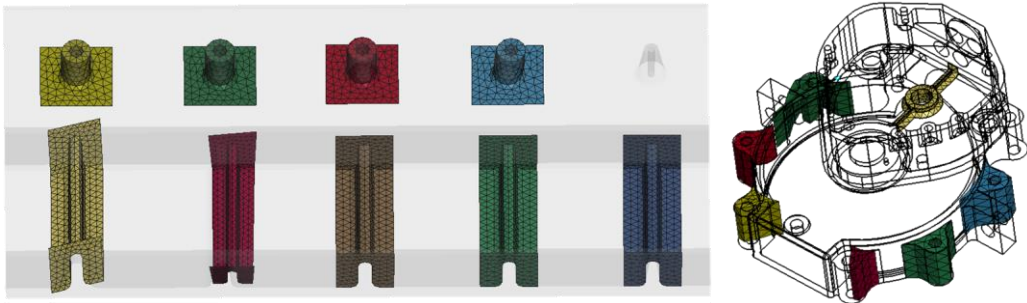
Figure 9: Results of applying extracted FE meshes: (a) applying FE meshes using extracted similar ribs and bosses with simple shapes and (b) applying FE meshes using extracted complex features with anisotropic scale and multiple similar features.
