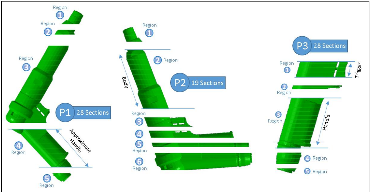
Figure 9: Segmentation results for the pistol-shaped drill illustrative example.
