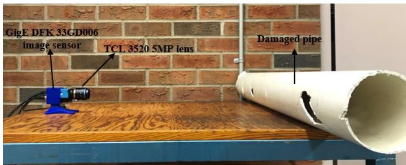
Figure 5: Dataset acquisition setup.
