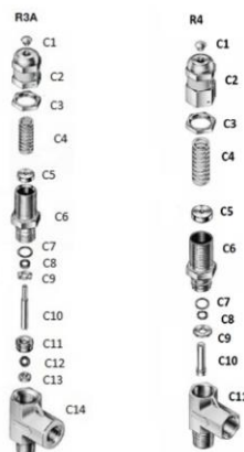
Figure 8: Exploded view of the new valve (R3A series) vs existing valve (R4 series) [25].
