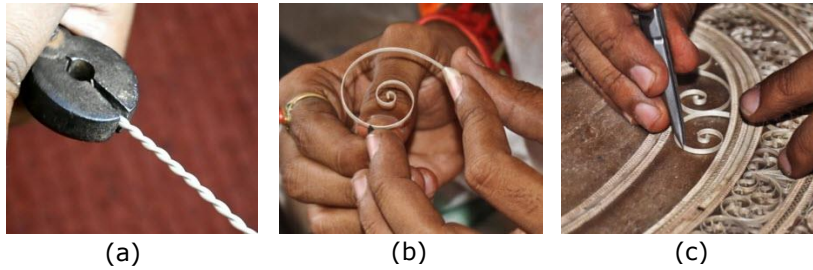
Figure 5: Conventional Method of (a) Making twisted wire strand (b) bending wire into motif shape (c) placing motif in a frame and soldering.
