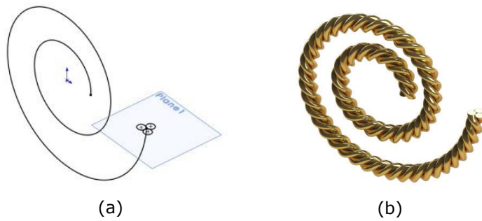
Figure 6: Figure 6: Modeling of twisted wire strand (a) plane for wire profile and sketching geometry (b) sweeping and twisting of wire profile (twisted wire strand made of 3 wires).
