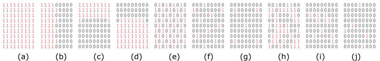
Figure 8: Target point distributions. '1' indicates where the surface control point is placed and '0' is where it is absent. (a) Full points. (b) Left half only. (c) Convex surface only. (d) Concave surface only. (e) 40 points evenly placed. (f) 10 points evenly placed. (g) 5 points evenly placed. (h) 40 points randomly placed. (i) 20 points randomly placed. (j) 5 points randomly placed.
