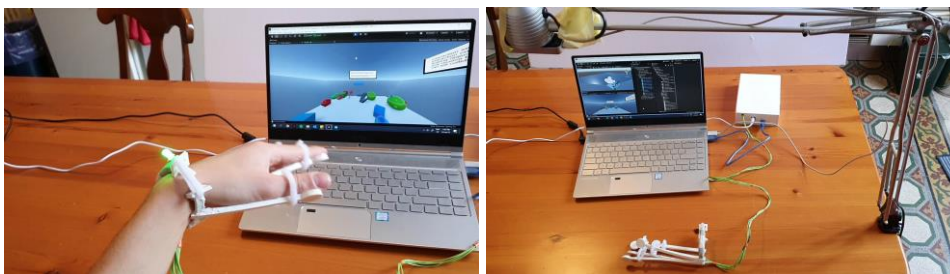
Figure 10: (a) haptic feedback glove in use (b) suggested setup.
