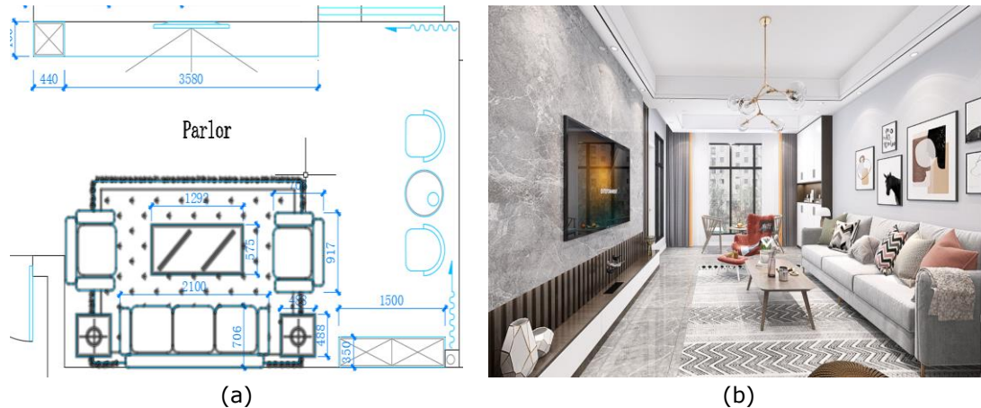
Figure 3: Floor plan and 3D rendering picture of the parlor: (a) floor plan of the designed parlor; (b) 3D rendering picture of the parlor.
