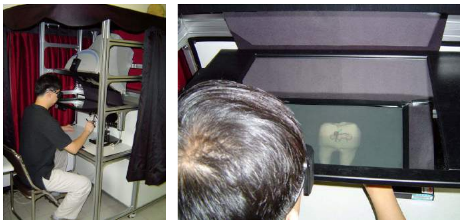
Fig. 10. Multi-modal Workbench. The user views images on the mirror.
