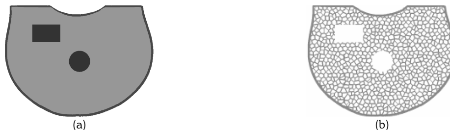
Fig. 7. (a) The design intension adding on the trabecular bone area shown in the middle. (b) The reconstructed vertebrate model with the designed feature, a circular and rectangle holes.
