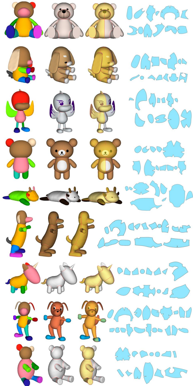
Figure 11: Some examples of pattern design. (From left to right, each row shows the model with segmentation, structure lines, seam lines, and 2D patterns).
