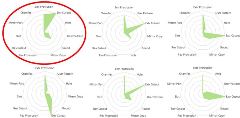
Figure 4: Examples of permuted Kiviati diagrams with FBC space and FBC profile for 11 feature types with 6 feature types considered in-scope features and 5 feature types considered out-of-scope features.
