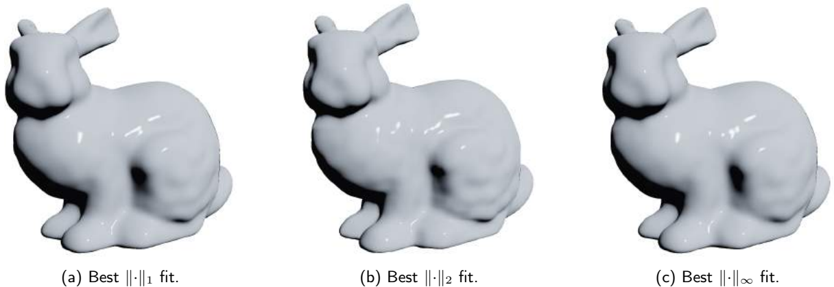
Figure 7: Comparison of best LSQ fits in different norms. The field is a second order DSDF with the resolution of 32 \times 32 \times 32 . Note the subtle differences in reflections. Since both visual and error metric results were similar, we chose \|\cdot\|_2 due to its simplicity and efficiency for field generation.
