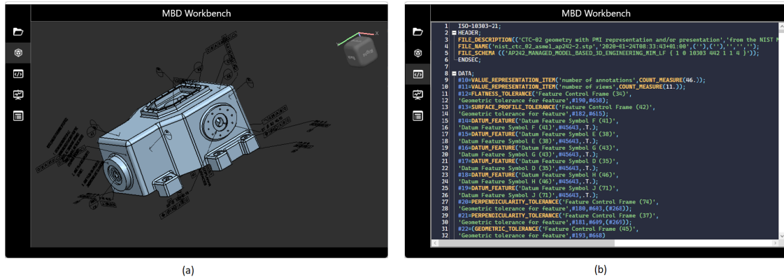
Figure 5: An example of using the program. A - module responsible for displaying the graphic representation of the model, B - preview module of the STEP file source code
