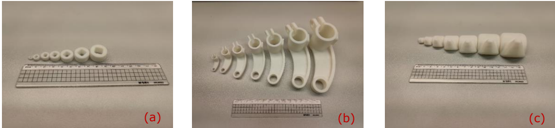
Figure 11: Pictures of 3 groups of parts, which are: (a) the simple part group, (b) the complex part group, and (c) the curved-surface part group
