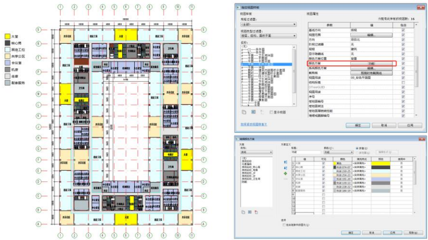
Figure 18: Colored floor plan generation and its color scheme setting.
