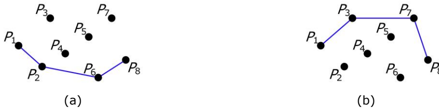
Figure 5: Compute convex hull based on the Andrew algorithm: (a) The lower half of the convex hull, (b) The upper half of the convex hull.
