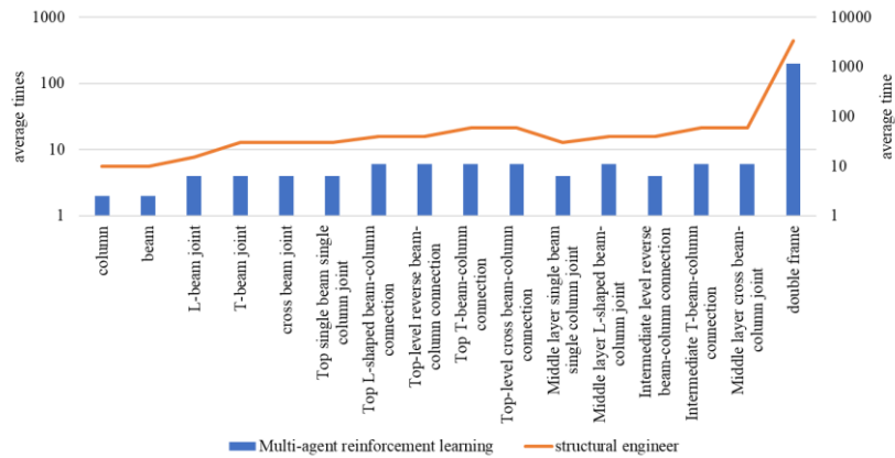
Figure 6: Comparison of the average time spent in the design of steel bars in reinforced concrete members (changed to a double column chart).
