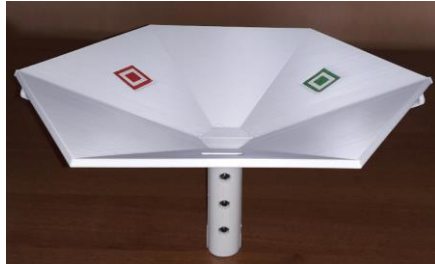
Figure 2: Specimen used to calibrate the mutual placement between the three depth cameras on the circular ring.
