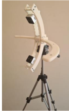
Figure 10: Ear scanner manufactured with Fortus F370 3D printer.
