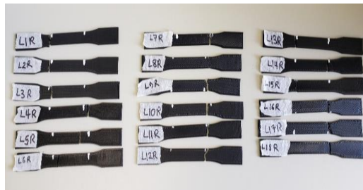
(b) Tensile samples after the test
