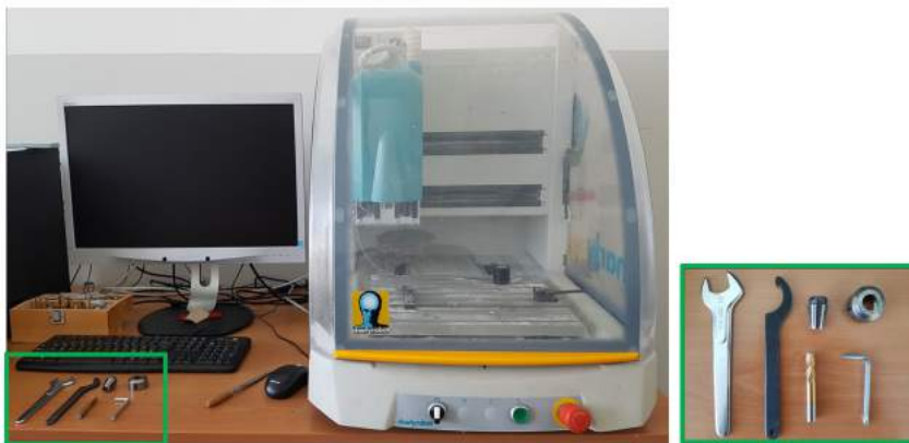
Figure 1: The Charly4U CNC milling machine and some of its associated tools
