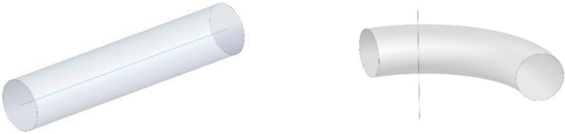
Figure 3: (a) Center line of a cylinder segment and (b) Axis of rotation of a non-cylindrical segment.
