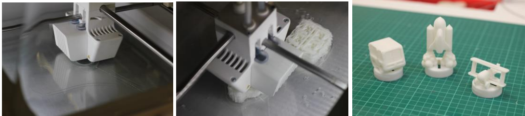
Figure 4: FDM Printing process of Capscoiner. From left to right. (a) 3D Printing of the Base, (b) Infill of the Pieces can be shown in the Process, and (c) Printing Pieces after Support Removal.
