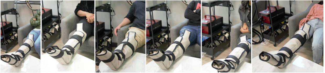
Figure 4: User-centered research – Fit testing the anthropometric research backed wrap prototype on volunteers from different ethnic backgrounds and UK foot size ranging from 4 to 12 (representative of the 5 th to 95 th percentile population in the world).
