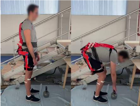
Figure 1: Operating principle of a low-back exoskeleton based on backbone kinematics.
