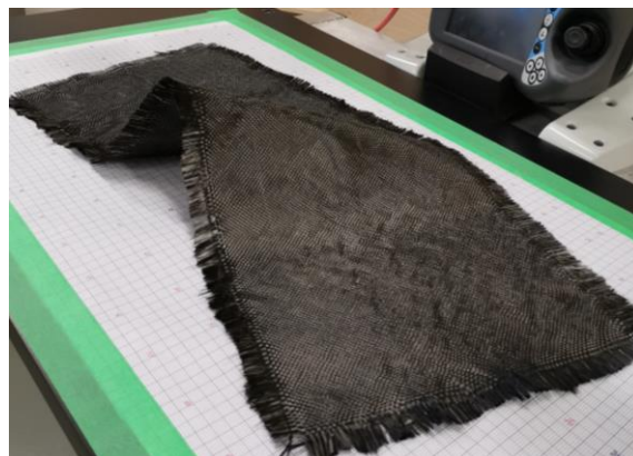
Figure 4: An example of wrinkling after fabric placement; adapted from [2].
