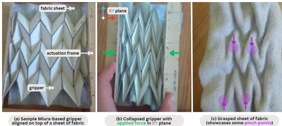
Figure 20: Potential actuation approach for Miura-based gripper using a frame, adapted from [29].
