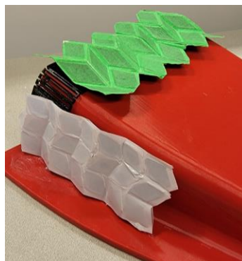
Figure 27: Two Miura-fold gripper connected with an Origami-based living hinge connector showcasing conformity over the composite mold.
