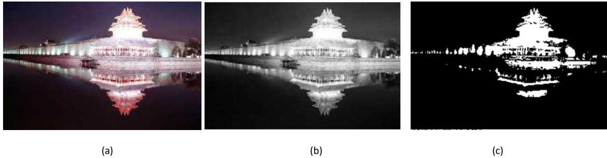
Figure 1: (a)Original Image, (b)Diffuse Reflection Part, (c)Specular Reflection Part.
