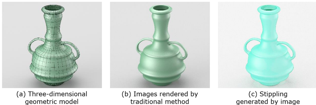
Figure 4: A stippling sketch is generated from an image rendered by a 3D entity.
