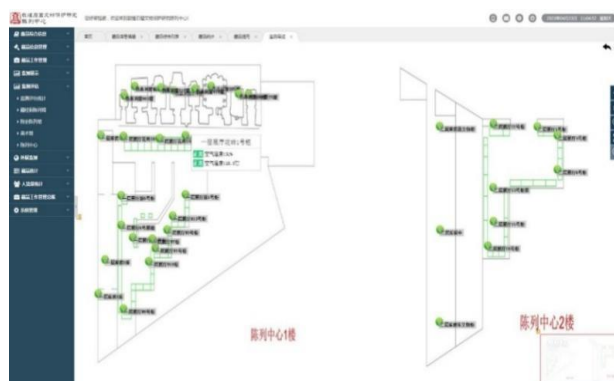
Figure 13: Monitoring (temperature and humidity) navigation interface.
