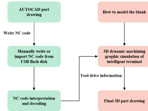
**Figure 1:** General structure of NC lathe machining simulation system.
