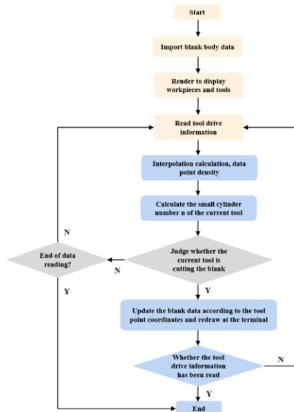
Figure 2: Dynamic turning process flow chart.
