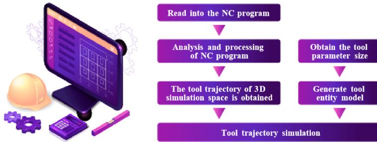
**Figure 4:** Simulation process of tool motion path.
