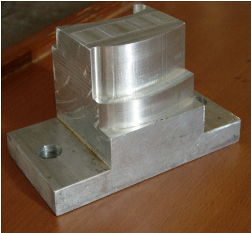
Fig. 5. Machined Parts for Shape Matching (A Logarithmic Spiral).
