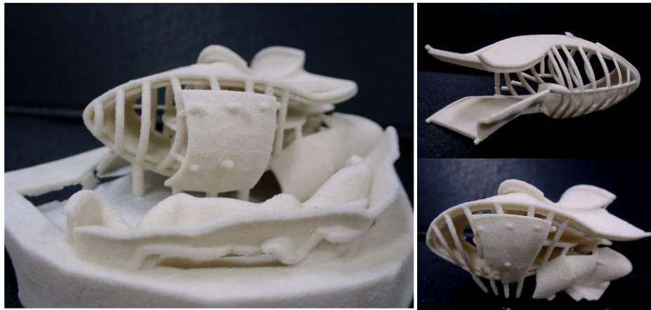
Fig. 3 Design interpretation (left) and RP parts (right).
