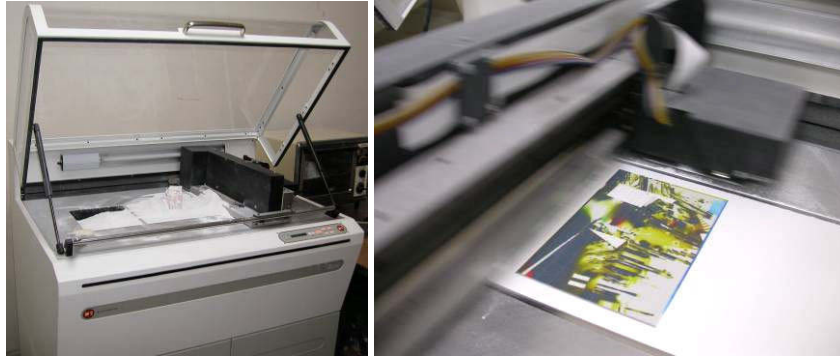
Fig. 1. The layering type RP machine (left) and a color printing in process (right).
