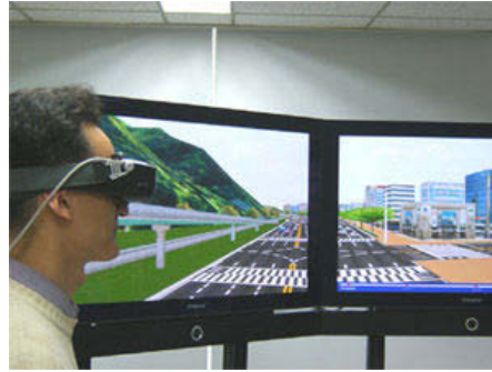
Fig. 7. Stereoscopic vision with wearing a head mounted display device.
