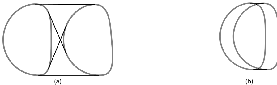
Fig. 3. (a) Two disjoint planar convex shapes have four bi-tangents. (b) Two intersecting planar convex shapes can have two bi-tangents only.
