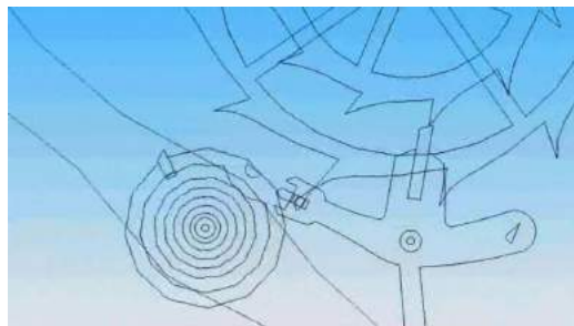
Fig. 10: The wire-frame model of the Daniels co-axial double-wheel escapement.
