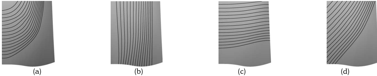
Fig. 1: (a) Surface with small local irregularities those are recognizable by circular highlight lines. In this figure, (b), (c), and (d) show that it is difficult to detect surface irregularities using conventional highlight lines.
