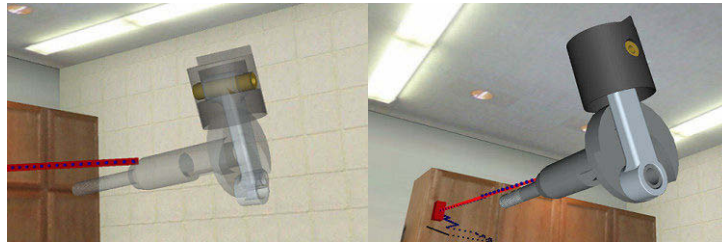
Fig. 9 (left): Crankshaft is being manually attached to piston assembly in a virtual demonstration, Fig. 10 (right): Automatically adjusted placement of crankshaft after motion smoothing.
