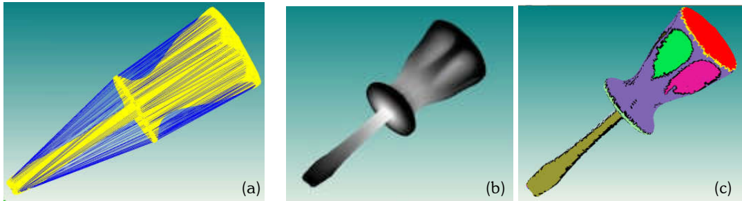
Fig. 1: (a) A point cloud of a screwdriver and its convex hull, (b) The screwdriver point cloud concavity intensity map (c) Different regions detected by the region growing method.
