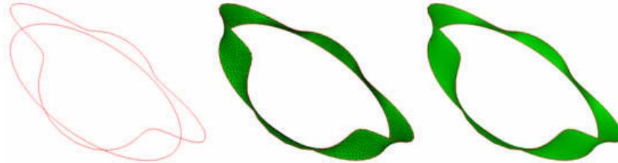
Fig. 9: Left: two input contours; middle: the resulting mesh; right: the shading image.
