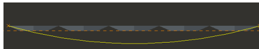
Fig. 26: The bending profile corresponding to the cavity shape of middle part of mould.
