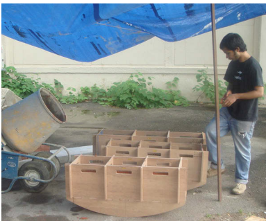
Fig. 9: Rocking mechanism for curing blocks.
