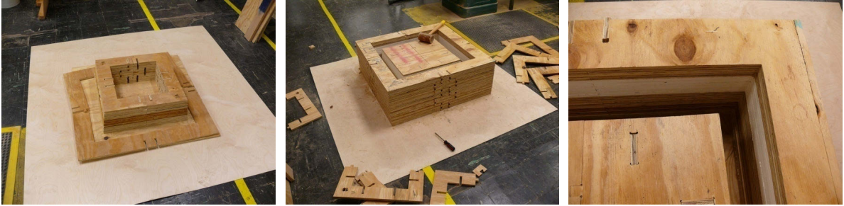
Fig. 7: CNC routed mold of 2'-0"x2'-0"x2'-0" (2" perimeter thickness) hollow cube.
