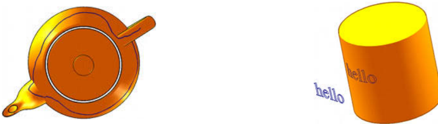
Fig. 1: The left image shows a single curve sketched over several surfaces all around by interleaving the sketching process with scene's transformations. The right image presents a precise projection of a group of curves over a cylinder.
