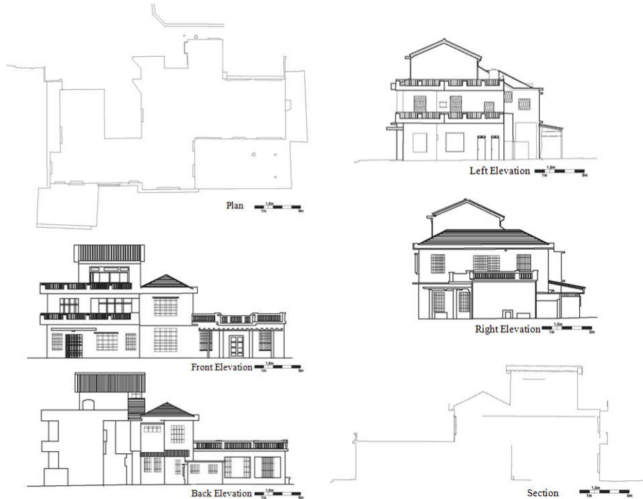
Fig. 6: Drawings generated by tracing point clouds.
