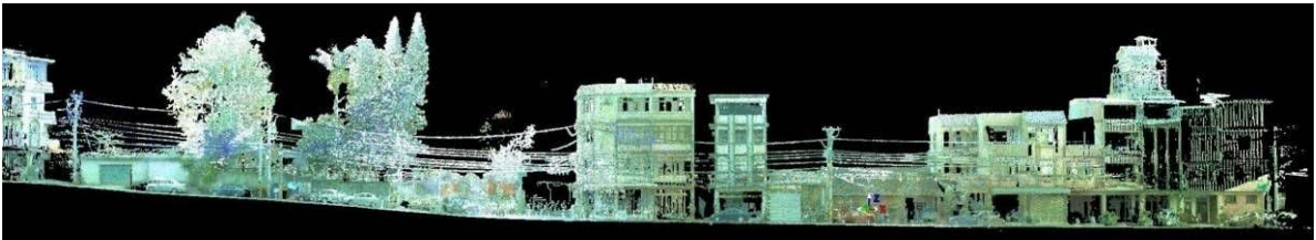
Fig. 4: Elevations of the entire street presented by point clouds.
